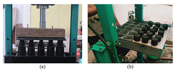
Figure 2. One of the stages of making briquettes: (a) dough pressing; and (b) printed briquettes
