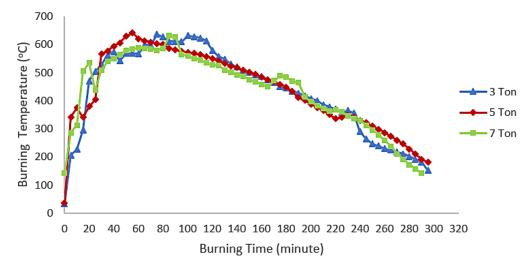
Figure 5. Burning time to ashes from rice husk charcoal briquettes of different compacting pressures
