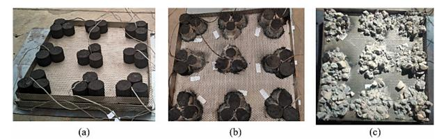
Figure 4. Changes in conditions of rice husk charcoal briquettes at different compacting pressures during combustion testing: (a) initial conditions; (b) briquettes start to smolder; (c) briquette burning ash
