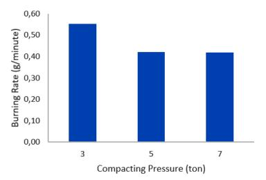
Figure 6. Burning rate of rice husk charcoal briquettes at different compacting pressures
